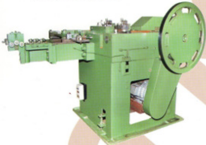
WIRE NAIL MAKING MACHINE
