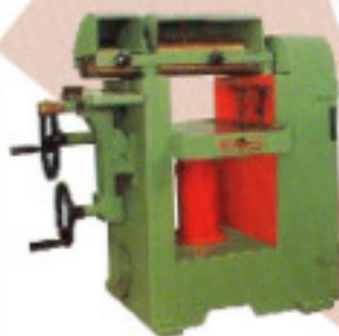
CLASSIC SERIES THICKNESS PLANNER - Piston Type
