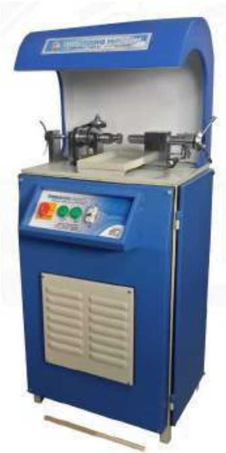
Threading Machine - For Making Tube Earring Post
