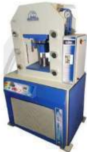
Hydraulic Press For Coin Pressing
