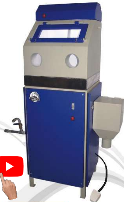
25.0401 and 25.0411 Water Jet for Casting Tree Cleaning - With Italian Pump Inside - Available SS Body and PP Body
