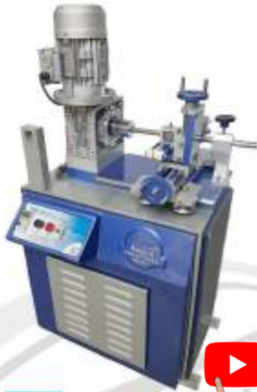
16.0431 Electric Tube Forming Machine - With Speed Controller AC Drive - With Italian Motor & Italian Gear Box
