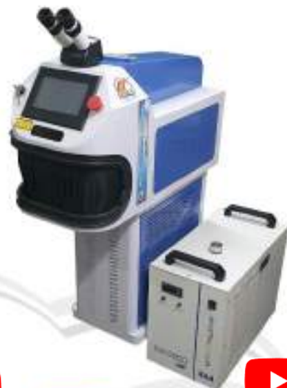
48.1233 Eagle Laser Welding Machine - Available 230W
