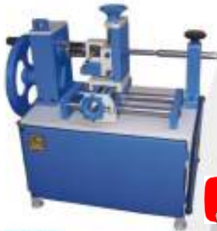
16.0301 Manual Tube Forming Machine - Hand Powered with Gear Box - Big Model Also Available for Quick Production
