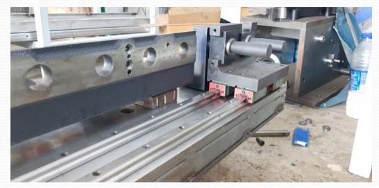
Hole CD Checking Gauge (1800 mm L)
