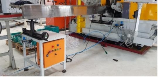
Suspension Rod/Shaft Loading & Unloading Conveyor
