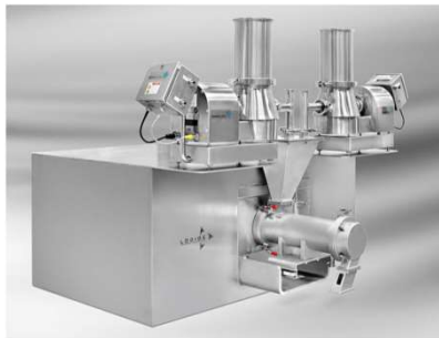
Continuous Granulator KM-5 with weigh feeders
