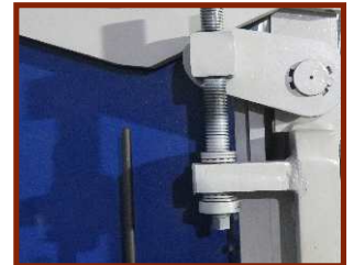
Ram Tilting Arrangement to Maintain bending over a period.
