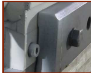
Manual Anti deflection setting for upper punch.
