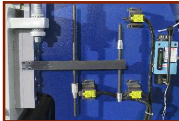
Limit Switch Assembly with Micro Setting for repeat accuracy
