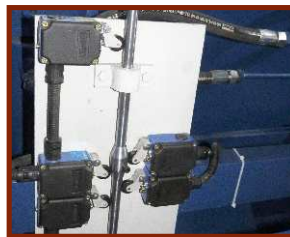
Variable Rake Angle Limit Switch Adjustment For Higher Thickness Cutting than nominal Capacity.
