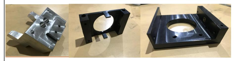
CNC milling allows us to quickly and accurately machine your parts from the stock material of your choice, in either metal or plastic. Critical shapes are easily created to a high standard of accuracy and surface finish. Tool and job presetting help to insure fast turnaround and accuracy. We use high end milling machines indulging 4 axis Capabilities.
