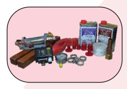
Furnace coil insulation materials Hardener, base, FRP tape, Silicon tape, Parmali support, FRP sheets etc.
